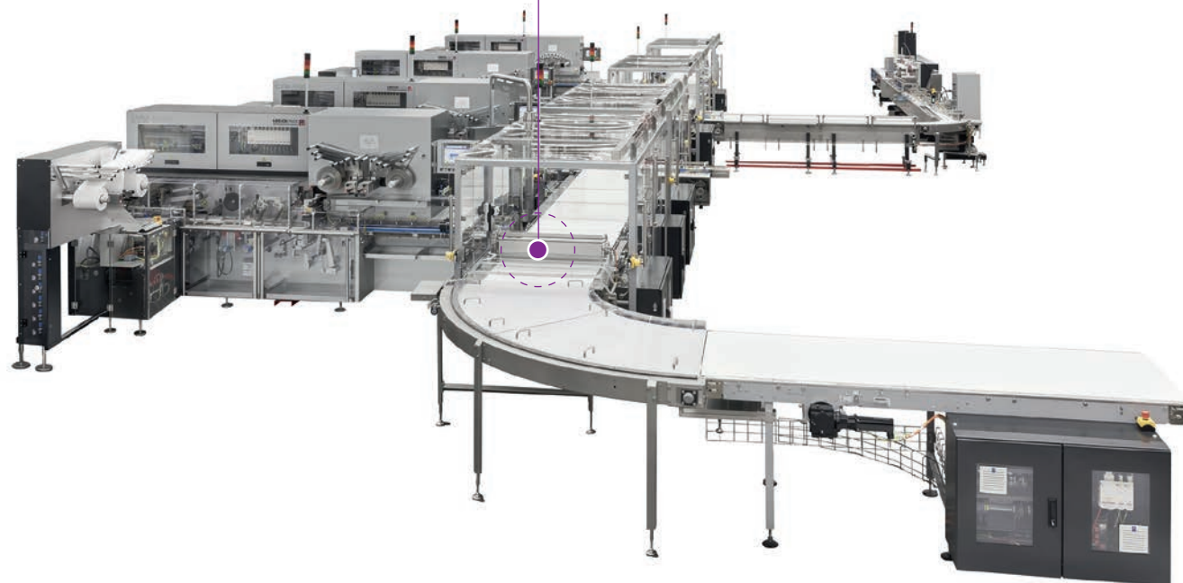
LOMATIC with four discharge stations, both directions being possible in the same discharge.
